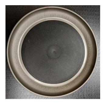
• If the poppet on the bottom of the base is missing or damaged, the base should be removed from service. Visually inspect the poppet to ensue it is not damaged or missing. If water or steam escape from the poppet during activation, this also indicates damage and the base should be removed from service.
